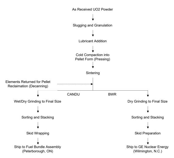
Figure 2: Uranium Fuel Pellet Manufacturing Process
