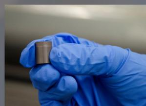
In Toronto, we manufacture ceramic pellets from natural uranium dioxide powder. After pressing, baking, grinding and inspecting the pellets, we send them to our Peterborough facility where they are placed in CANDU® fuel bundles. The fuel bundles are then sent to Ontario Power Generation's Darlington and Pickering Nuclear Generating Stations. Both our Peterborough and Toronto facilities are licensed by Canada's nuclear regulator, the Canadian Nuclear Safety Commission (CNSC).
