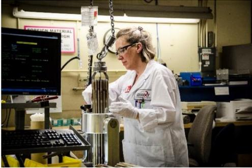
Fuel manufacturing operations involve the loading of fuel pellets into Zircaloy tubes, sealing, and welding of the tubes to produce fuel elements and the assembly of the fuel elements into fuel bundles. The basic assembly process is described in Figure 2.
